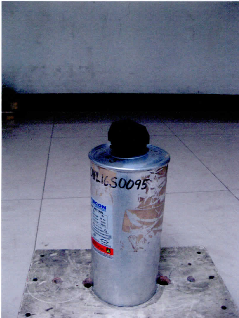
Photograph- 1: A view of the test capacitor on completion of destruction test
